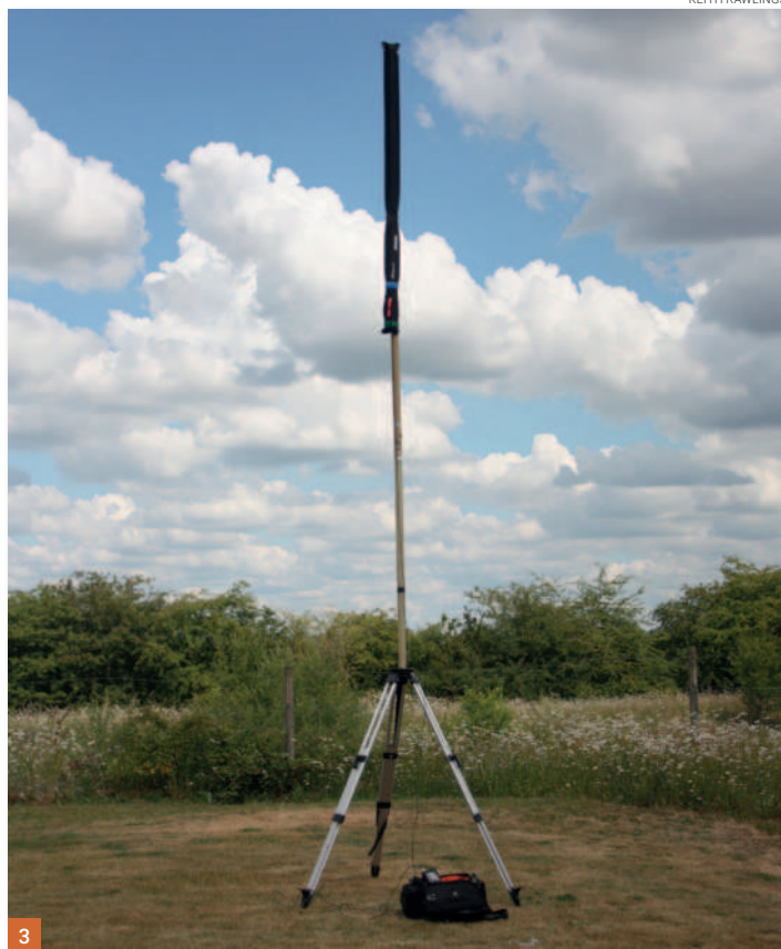
Fig.1: The Black Knight antenna inflated, with a camera bag. Fig. 2: Black Knight folded up, with a camera bag. Fig. 3: The Black Knight on a tripod mast at my 'test range'. Fig. 4: The Black Knight Standing Wave Ratio (SWR) and Impedance Plot. Fig. 5: AN-SOF medium wave broadcast aerial simulation. This demonstrates power density (above) and current distribution (below).
