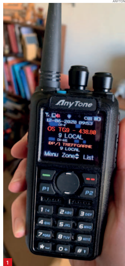
Fig.1: An Anytone DMR handset, mainly used by radio amateurs.
